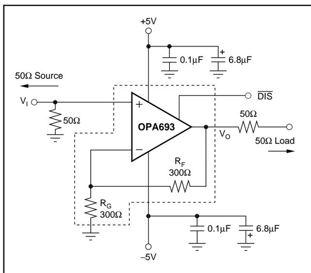
Figure 1. DC-Coupled,  $G = +2$ , Bipolar-Supply, Specification and Test Circuit.
