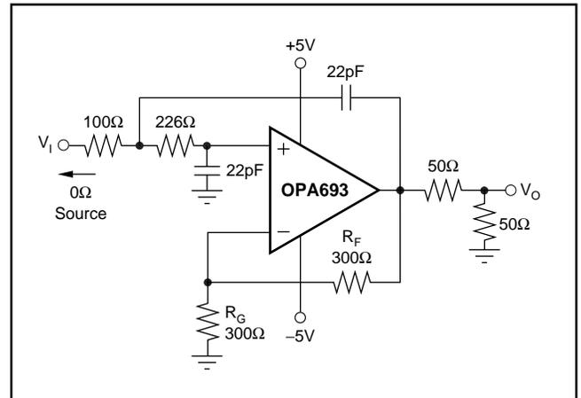
Figure 10. Line Driver with 40 MHz Low-Pass Active Filter.
